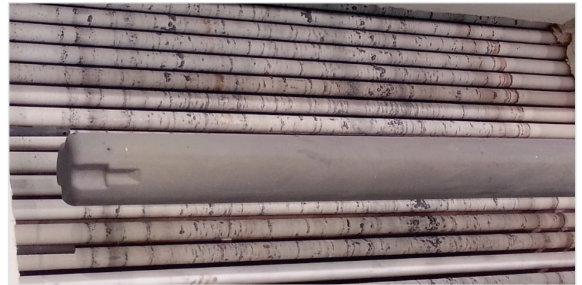
Image of ZYAROCK® HoSt-M™ rollers after 6 months operation time with about 160.000 AISi coated steel blanks transported.
